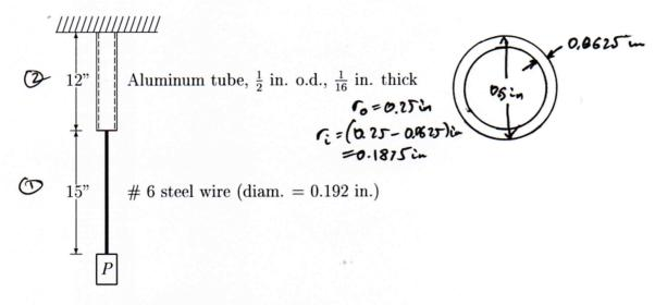
$$E_{\rm steel} = 30 \times 10^6 \text{ psi}, \qquad E_{\rm Al} = 10 \times 10^6 \text{ psi}$$
