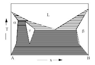
(a) Only the one-phase fields are shown in the phase diagram above. Outline and label the two-phase fields.
