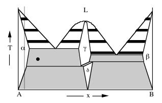
(a) A possible state of the system is indicated by the dot on the left-hand side of the diagram. Give the phases present, estimate the compositions of the phases, and estimate their fractions when the system is at equilibrium in the state shown by the dot.
