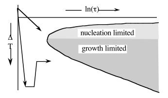
(a) If the material is cooled as indicated by the upper arrow, the final microstructure contains nuclei of  $\beta$  almost exclusively in the grain boundaries of the  $\alpha$  grains. Why might you expect this?
