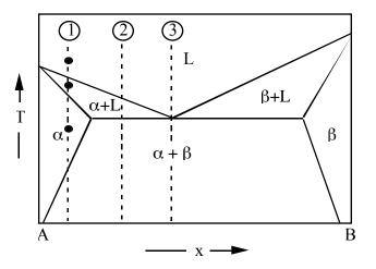
(a) Give the phases present, their compositions and their mole fractions at each of the three points indicated by dots in the phase diagram. (Assume an overall composition x = 0.1 and give plausible estimates for any other compositions you need.)
