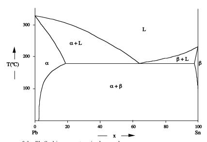
The phase diagram of the Pb-Sn binary system is shown above.
