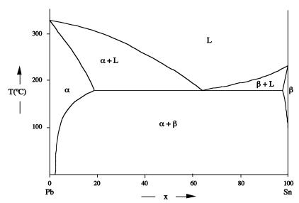
The phase diagram of the Pb-Sn binary system is shown above.
