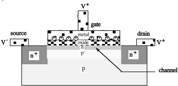
This figure shows a typical configuration of a metal-oxide-semiconductor field effect transistor (MOSFET). The drawing shows a positive voltage at the metal gate, which activates the inversion layer, or channel, in the underlying semiconductor.
