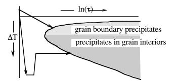
If the material is cooled as indicated by the upper arrow, the final microstructure contains nuclei of  $\beta$  almost exclusively in the grain boundaries of the  $\alpha$  grains. Why might you expect this?
