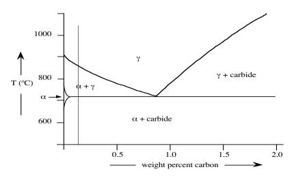
A portion of the Fe-C phase diagram is shown above. Suppose you are given a sample with about 0.2 wt.% carbon (the composition of the vertical line drawn in the figure).
