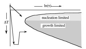
If the material is cooled as indicated by the upper arrow, the final microstructure contains nuclei of  $\beta$  almost exclusively in the grain boundaries of the  $\alpha$  grains. Why might you expect this?
