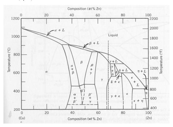
The Cu-Zn phase diagram is shown above.
