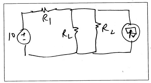
(b) Find an expression for the voltage recorded by the voltmeter in terms of  $R_1, R_2, R_L$ .
