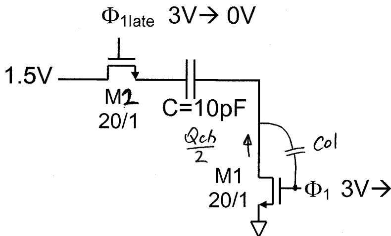
In the sampling circuit above, find the total sampling error for a sampling time of  $t_s = 2.5\text{ns}$ . Assume fast gating and 50% charge split. Hint:  $e^{-4} \sim 0.02$ .
