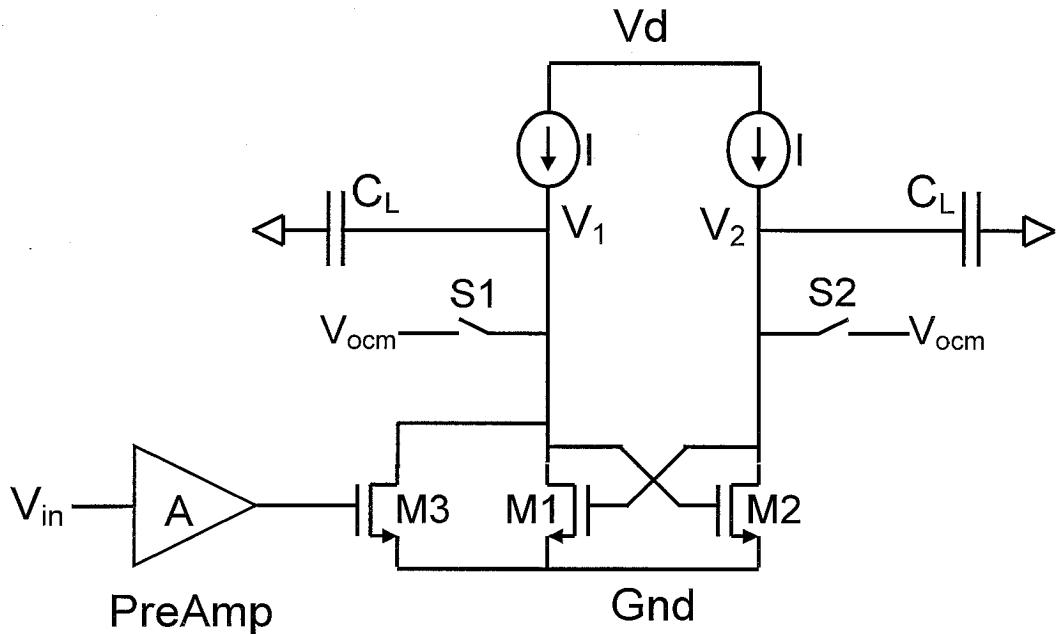
In the comparator circuit shown above,  $V_1$  and  $V_2$  are initialized to  $V_{ocm}$ . Due to the implementation errors switch  $S_2$  introduces an offset voltage of  $V_{os}$ . Given the offset voltage  $V_{os}$ , what is the minimum  $V_{in}$  that this comparator can successfully detect?
