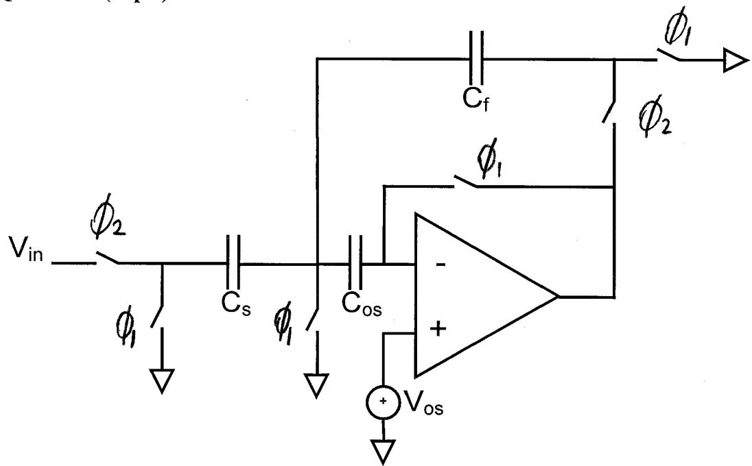
In the switch cap gain circuit above, there are two non-overlapping phases available:  $\Phi_1$ ,  $\Phi_2$ . In order to have an inverting gain stage with offset cancellation, assign appropriate phases ( $\Phi_1$  or  $\Phi_2$ ) to switches in the circuit.
