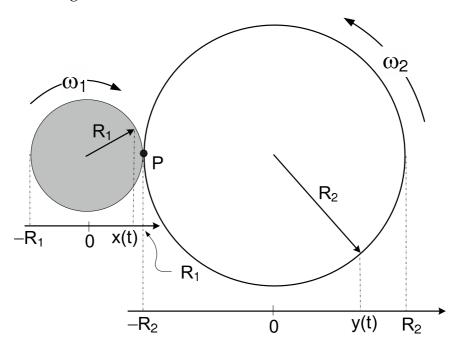
The respective radii of the two gears are shown in the diagram, and are related according to  $0 < R_1 < R_2$ .
