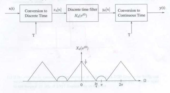
(a) Plot the spectrum of the continuous time signal x(t) (i.e., plot  $X(j\omega)$ , the CTFT of x(t)). Assume the continuous to discrete time conversion is ideal.
