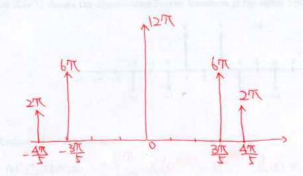
(c) The signal x(t) is now the input to an LTI system, whose frequency response  $H(j\omega)$  is given by  $\angle H(j\omega) = -2\omega$  and  $|H(j\omega)|$  shown in the following figure.
