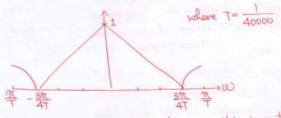
Note: This is in CTFT domain, this is not 2TR periodic. (b) We want to filter x(t) to keep only the lowpass component between 0 and 10 kHz, i.e., we want y(t) to represent the lowpass component of x(t). Plot the spectrum of the filter H<sub>d</sub>(e<sup>jΩ</sup>) needed to accomplish this task. Assume that the discrete to continuous time conversion is ideal.
