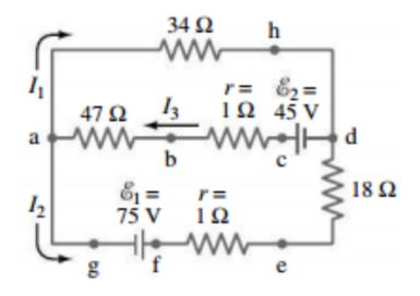
(a) [2 points] Using Kirchhoff's Loop Rule, derive an equation in terms of  $I_1$ ,  $I_2$  and  $I_3$  from the upper loop. Combine similar terms in your equation.
