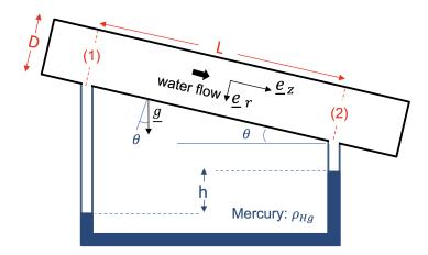
(a) (9 points) What is the pressure difference between section (1) and (2), i.e.  $(P_1 - P_2)$ , in terms of known variables? Note: The pressure does not vary radially within the pipe.
