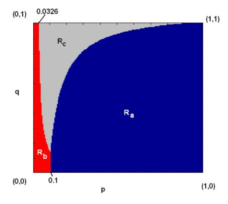
If the defective probability is too high (p very big), you should just throw it away. If the defective probability is too low, you should just send it to the customers. Otherwise, you should test the chip if the test is good enough (q reasonably big).
