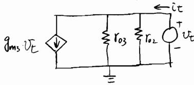
$$\Rightarrow Rout = \frac{UE}{\overline{L}E} = \frac{1}{3m_3 + \frac{1}{62/(703)}} = 2.2 \text{ K}\Omega$$
