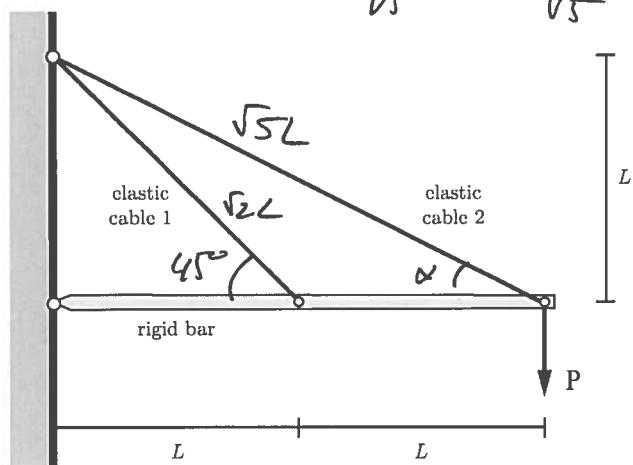
Statically indeterminate  $\Rightarrow$  Force method (3 steps)
