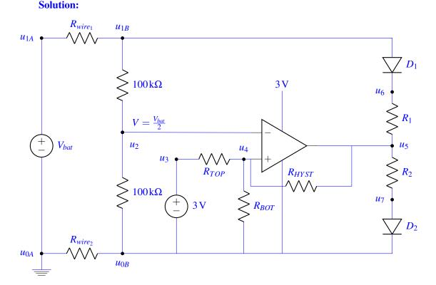
We solve this circuit with superposition, first setting the 3 V source to 0 V, and then setting the output of the comparator to 0 V:
