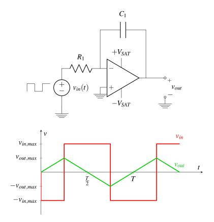
(a) Assume that  $v_{in}$  is an ideal voltage source that outputs a square wave with amplitude  $v_{in,max} = 5 \text{ V}$  and period T = 2 ms, and recall that  $v_{out}$  will be a triangle wave with peak value  $v_{out,max}$ . Both waveforms are plotted in the diagram above. If  $R_1 = 2 \text{ k}\Omega$ ,  $C_1 = 3 \text{ \mu}\text{F}$ , and  $V_{SAT} = 5 \text{ V}$ , what will be the peak value  $v_{out,max}$  of our output?
