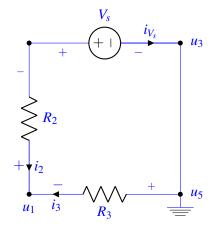
$$i_b = \frac{V_s}{R_3 + R_2} = \frac{4V}{2\Omega + 3\Omega} = 0.8 \text{ A}$$
