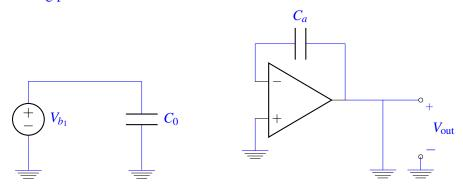
Capacitor  $C_0$  charges from the voltage source:  $Q = V_{b_1}C_0$ . With  $\phi_1$  closed,  $V_{out}$  is shorted to ground, and therefore  $V_{out} = 0 \text{ V}$ .
