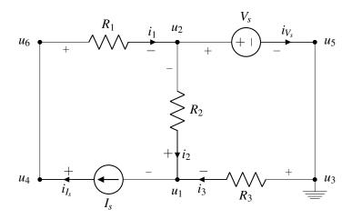
(d) Write the KCL equation for the currents associated with node  $u_2$  in terms of  $i_1$ ,  $i_2$ ,  $i_3$ ,  $i_4$ ,  $i_{I_s}$  and  $i_{V_s}$ .
