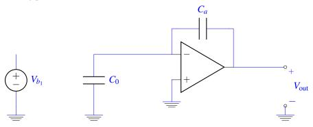
The charge Q from phase 1 is now shared between  $C_0$  and  $C_a$ :
