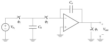
During phase 1,  $\phi_1$  is closed and  $\phi_2$  is open. During phase 2,  $\phi_1$  is open and  $\phi_2$  is closed. What is the voltage  $V_{out}$  during phase 1 and phase 2? You can assume that a long time has passed in each phase before  $V_{out}$  is measured.
