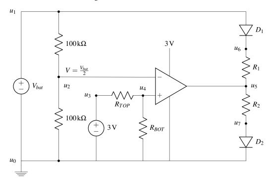
The green LED operates with a forward voltage,  $V_{f,grn} = 2.5 \,\text{V}$ , and current  $I_{f,grn} = 100 \,\text{mA}$ , so we need to determine the value of its current limiting resistor  $R_{GRN}$ . Similarly, the red LED operates with a forward voltage,  $V_{f,red} = 2.5 \,\text{V}$ , and current  $I_{f,red} = 50 \,\text{mA}$ , so we need to determine the value of its current limiting resistor  $R_{RED}$ .
