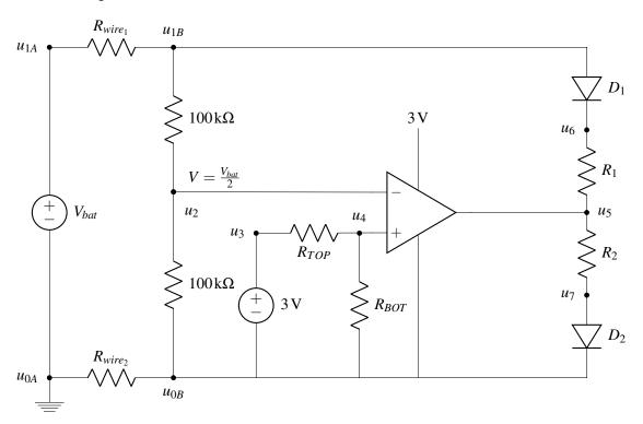
You suspect that there might be a sudden change in the voltage drop across these wires that reduces the voltage (nominally  $\frac{V_{bat}}{2}$ ) at the  $V^-$  input of the comparator when toggling between the two LEDs. Ignoring any hysteresis provided by the comparator, you decide to add your own hysteresis to try to solve the flashing problem.
