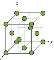
Sketch all of the atoms within the unit cell as described in (b). Specify the lattice and motif. Lattice = face-centered tetragonal Motif = one In atom per lattice point
