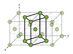
(d) What are the indices of the first diffraction peak from a simple tetragonal structure with the same parameters as indium? (HINTS: Bragg's Law applies, that is,  $n\lambda = 2d \sin\theta$ , and all reflections are "allowed" by structure factor rules.) Ans: \_\_001\_\_
