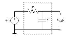
Figure 5: RC circuit that you suspect is inside the mystery (?) box.
