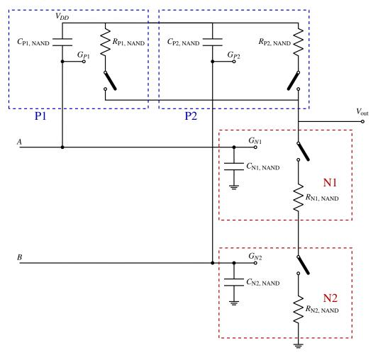
Figure 8: NAND Model: Capacitances
