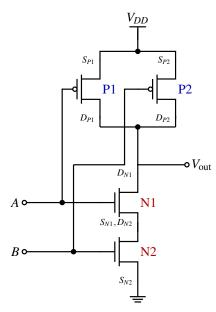
(a) NAND schematic with transistors.
