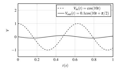
Figure 11: Input-Output behavior of the filter Divija built.
