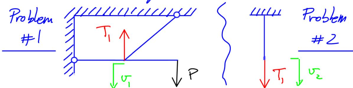
**STEP 2** Solve for the deflections  $v_1$  and  $v_2$
