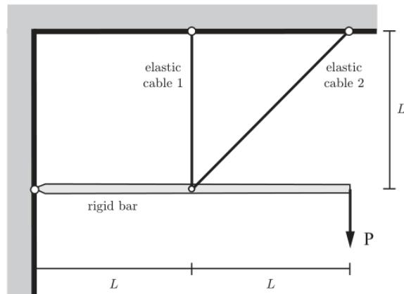
*Statically indeterminate  $\Rightarrow$  Force method (degree of indeterminacy = 1)*
