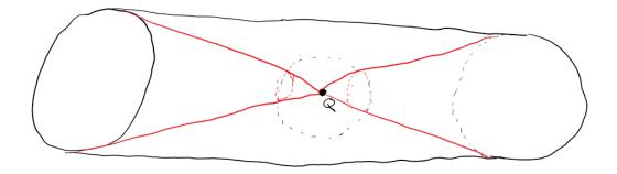
The advantage of this method is that it is much easier to calculate the flux through a portion of the sphere, since the electric field of a point charge is constant around a spherical surface. The total flux is given by Gauss's law as  $\Phi_{\text{total}} = Q/\epsilon_0$ . Since the radius and half-length of the cylinder are both  $R_0$ , we get a cone-angle of  $\pi/4$ . We can calculate the portion of the area of the sphere this takes up like so:
