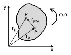
$\underline{\mathbf{a}}_{\mathrm{P}} = \underline{\mathbf{a}}_{\mathrm{A}} + \underbrace{(\underline{\alpha} \times \underline{r}_{P/A})}_{\mathbf{a}_{\mathrm{tangential}}} \underbrace{-(\omega^{2}\underline{r}_{P/A})}_{\mathbf{a}_{\mathrm{radial}}} \qquad (\text{Relative acceleration between two points on a rigid body})$   $\underline{\text{Moment Balance about center of mass, cm}}$
