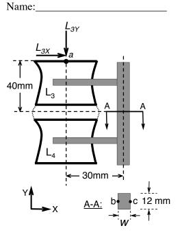
(iv) [8 points] Write out an expression for the normal stresses in the Y-direction for points b and c at section A–A in terms of W,  $L_{3Y}$  and  $L_{3X}$ .
