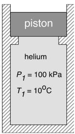
As shown at left, a piston and cylinder device whose piston is resting on a stop contains 0.5 kg of helium gas, initially at 100 kPa and 10°C. The mass of the piston and the effect of the atmospheric pressure acting on the piston are such that a pressure of 500 kPa is required to raise the piston off the stop.
