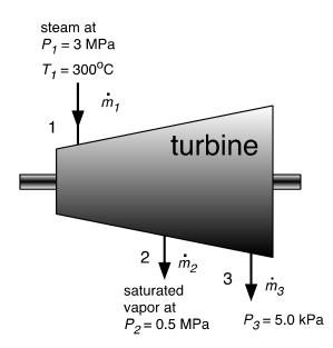
A well-insulated (adiabatic) turbine operating at steady state with steady inlet and exit conditions is shown schematically above. Bulk kinetic and potential energy
