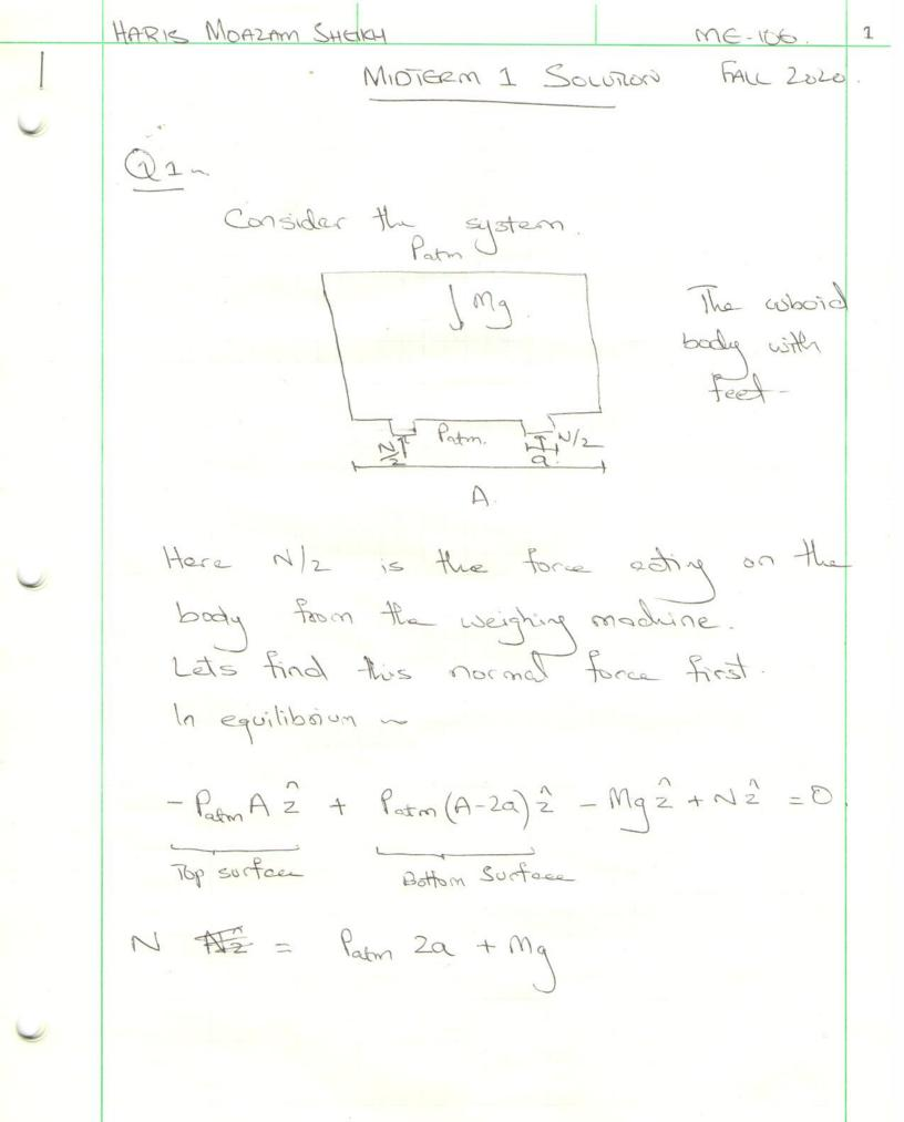
2 The total force acting on the weighing moduline Dis. -102 (W) = Mg + Patm 2a + Patm (A-2a) force by body force due to air pressure. 1601 = Mg + Palm A. (c) is independent of a.
