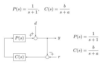
Design the controller parameters a, b such that
