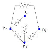
Use the minimization principle explained in class to calculate the voltages at the nodes  $n_1, n_2$ .
