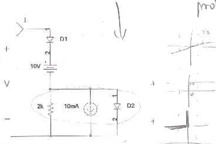
Using the grid shown below, plot the I-V graph of the circuit above. Assume all diodes are ideal.
