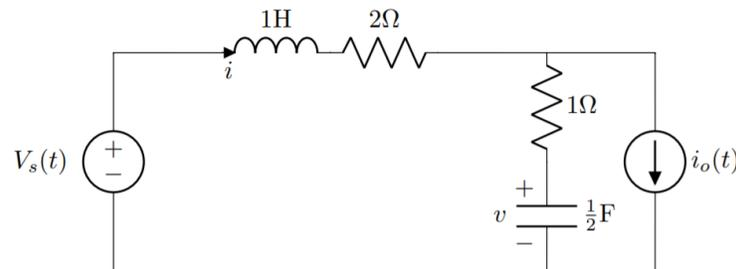
MB3. Consider the circuit above with the inductor current and capacitor voltage as state variables.
