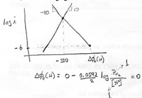
(a)  $\therefore$  Kinetics of reduction of  $H^+$  on Fe in 1M HCl are described by
