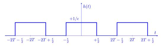
h(t) is periodic with fundamental period 2T and fundamental frequency  $2\pi/(2T) = \pi/T$  (like g), and its Fourier series decomposition is:
