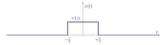
The output signal will be y(t) = (g \* x)(t). g(t) can be written as a linear combination of x(t):
