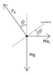
Notice that the slope of the surface of the water is equal to  $\tan \theta$  (rise over run). If we find the slope of the surface of the water as a function of R,
