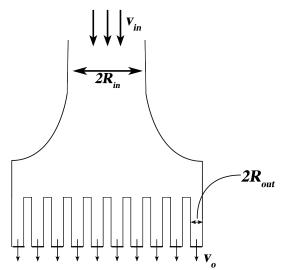
b) Derive an equation for the outlet velocity  $(v_o)$  of an outlet nozzle in terms of inlet velocity  $(v_{in})$ , the number of nozzles *n*, inlet and outlet radii  $R_{in}$  and  $R_{out}$ , and any other material parameters needed. Leave all quantities as variables and write your final answer in the box provided below. (10 points)
