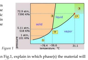
a) Based on the phase diagram shown in Fig.1, explain in which phase(s) the material will be when it reaches thermodynamic equilibrium with its environment.
