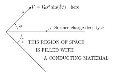
An infinite conducting wedge has an opening angle of  $\pi/4$ .
