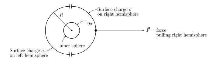
A sphere of radius R is carrying a uniform surface charge density  $\sigma$ . Inside it is an smaller sphere of radius R/3 carrying (an oppositely charged) surface charge density  $-9\sigma$ . The outer sphere is cut in half, and the two hemispheres (left and right) are separated, with a very (infinitesimally) thin gap between them.
