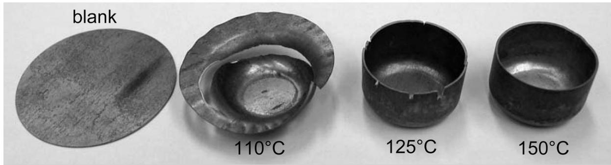
**Figure 2-1** Results of deep drawing a Mg-3 wt.% Al 1 wt.% Zn alloy as a function of temperature. From S.R. Agnew, J.W. Senn, and J.A. Horton, *Journal of Metals*, May 2006, p. 62.
