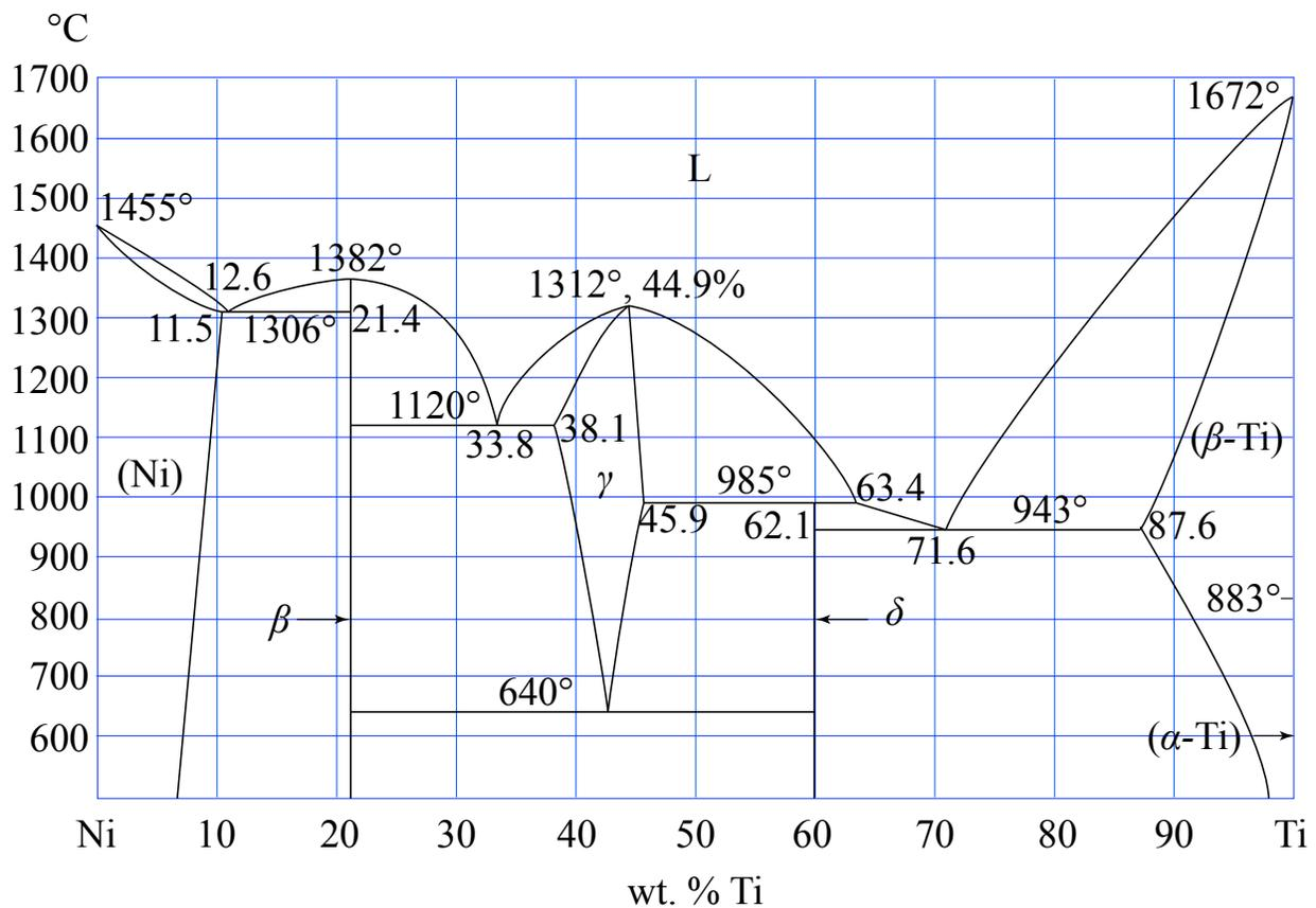
**Figure 1-1** The Equilibrium Nickel-Titanium Phase Diagram, from the *Metals Handbook*, Volume 8, 8<sup>th</sup> Edition, American Society for Metals, Metals Park, Ohio, (1973), p. 326.
