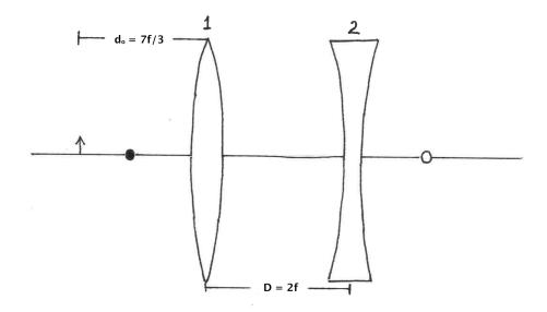
Two thin lenses, one converging and one diverging, are aligned horizontally. The two foci of the converging lens (number 1) are a distance f from its center; one such focus is shown by the filled circle. Similarly, the two foci of the diverging lens (number 2) are also a distance f from its center; the open circle shows one of these foci. The lens centers are a distance D = 2f apart.
