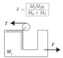
(b) The tension T has to balance  $M_3$  in the vertical direction, so  $T = M_3 g$ . But the same T also needs to pull  $M_2$  such that  $M_2$  has the same acceleration as the entire system, so  $T = M_2 a$ . Hence  $a = M_3 g/M_2$ . The force F that moves entire system  $M_1 + M_2 + M_3$  with acceleration a should have magnitude
