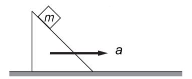
A 45° wedge is pushed along a table with constant acceleration *a*. A block of mass m slides without friction on the wedge. Find the block's acceleration relative to the ground. Gravity is directed down.
