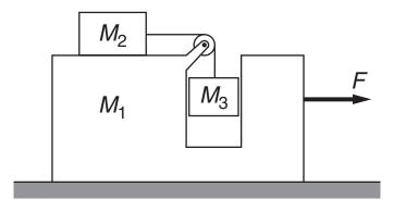
Consider a system of 3 masses, one pulley and one massless string as illustrated in the sketch. All surfaces are frictionless.
