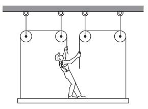
A painter of mass M stands on a scaffold of mass m (m<M) and pulls himself up by two massless ropes, which hang over pulleys, as shown. Ignore any friction.
