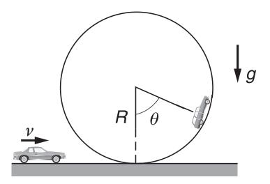
An automobile of mass *M* drives at constant speed *v* onto a loop-the-loop, as shown.
