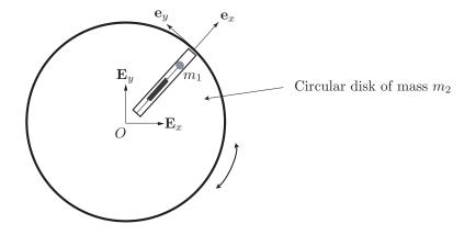
Figure 4: A particle of mass  $m_1$  is free to move in a smooth slot on a circular disk of mass  $m_2$ .
