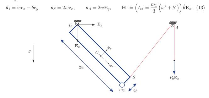
Figure 3: A rigid body of mass  $m_1 + m_2$  is free to rotate about O and is subject to a gravitational force.
