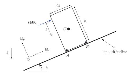
Figure 2: A crate being pushed up an incline by a constant force  $P_0 \mathbf{E}_x$ .
