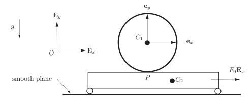
Figure 5: A rigid cylinder of mass  $m_1$  and radius R moving on a cart. A constant force  $F_0 \mathbf{E}_x$  acts on the cart.
