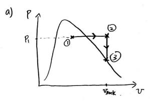
b). Initially, constant pressure heat addition. When V = Vent, constant volume heat removal.  $V_3 = V_2 = V_{evck} = \frac{V_{evck}}{m} = \frac{0.7m^3}{5kg} = 0.14 \frac{m^3}{kg}$ . • Find sat. T and P that  $V_q = V_{evck} = 0.14 \frac{m^3}{kg}$  $\Rightarrow \begin{bmatrix} P_3 = 1400 kPa, T_3 = 195.04^{\circ}C \end{bmatrix}$
