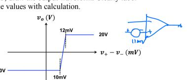
d) With the Op amp characteristics -20V 10mV shown in c), if the *open loop* 10mV bandwidth of the Op amp is 1 kHz, what is the bandwidth of the amplifier?
