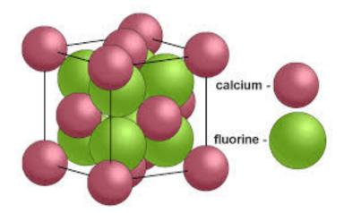
2. **[20 points]**  $CaF_2$  is a compound that forms ionically with the structure shown above. The Ca atoms are positioned on the sites of a cubic F-lattice. Each Ca atom is surrounded by 8 F atoms, positioned at the tetrahedral interstitial sites. The experimentally measured formation enthalpy (per formula unit) is:
