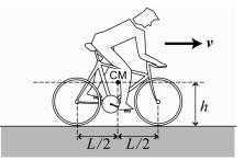
b) 10 Points. Find the relationship between h and L, the distance between the centers of the wheels, to keep the bicycle from overturning and throwing the rider over the handlebars.
