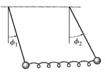
$L(\phi_2 - \phi_1)$ .] Write down the Lagrange equations of motion. (b) Find and describe the normal modes for these two coupled pendulums.
