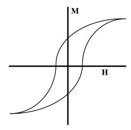
Simple ferromagnetic materials, like Fe, Ni and Co, are ferromagnetic at low temperature essentially because their atoms have net magnetic moments that align with one another.
