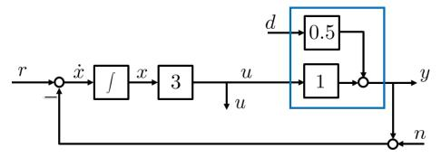
Fill in the 3  $\times$  4 matrix which relates (x, r, d, n) to  $(\dot{x}, y, u)$  as shown below
