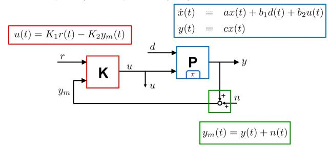
Keep the plant parameter a as a general value, but assume  $b_1 = b_2 = c = 1$ , for simplicity.  $K_1$  and  $K_2$  are gains (constants). Keep these as variables. Specific values will be designed in part (b) of the problem.
