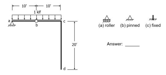
(b) State whether the truss shown is (a) unstable, (b) stable and determinate, (c) stable and indeterminate, or (d) none of the previous.
