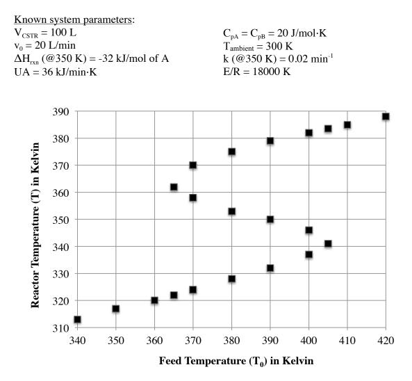
a) (2 points) Initially, you have a feed temperature of 400K. You increase it 15K and then drop it 35K. What temperature is the reactor operating at?
