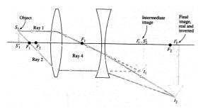
Generally, points are given for the second image if it is consistent with the first. The diagram each image. should show relevant features such as optic axis and focal points, and the standard rays used. Using the lens equation, with  $f_1 = +22cm$  (converging),  $o_1 = +32cm$  (real):
