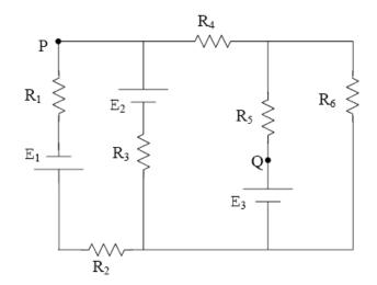
Figure 2: Resistor and Voltage Source Network.
