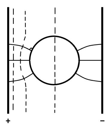
Where the solid lines are electric field lines and the dashed lines denote equipotential surfaces.
