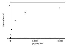
ANSWER: At 300K for  $\Delta G^{\circ} = \Delta H^{\circ} - T\Delta S^{\circ}$ = -9.5 kJ/mol - 300K \* 85 J/ (mol\*K) = -35 kJ/mol ⇒ $\Delta G^{\circ} = RT \ln K_D = -35 kJ/mol \Rightarrow K_D = 800 nM$ f<sub>bound</sub> = [L] / ([L] + K<sub>D</sub>) ⇒ 0.9 = [L] / ([L] + 800 nM) ⇒ [L] = 7200 nM
