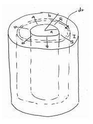
Now we can decompose this resistor as resistors (thin cylindrical shells) connected in series, cylindrical with radius  $a \le r \le b$ , length L, and thickness dr. Each shell has the resistance
