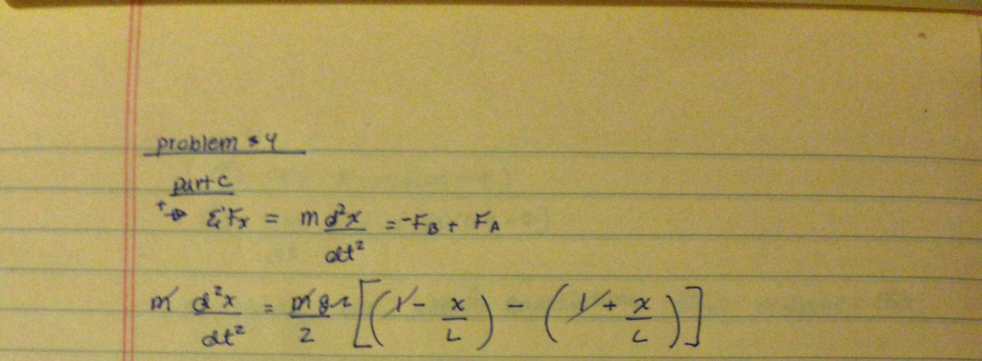
$\frac{d^2x}{dt^2} = -\frac{g_{12}}{2}\frac{\chi_2}{\zeta}$ or,  $\frac{d^2x}{dt^2} + \frac{rq}{L} x = 0$ 8 thas, we see me solution will be in the form of a simple harmonic oscillation since The ode takes the form dix + Ax = 0
